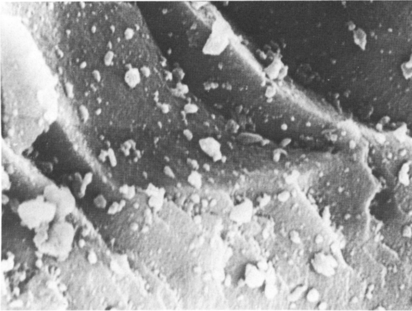
Fig. 3. Topography of carbon-silica adsorbent A 2 (SEM, \times 1000 ).
