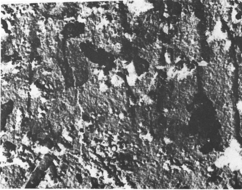
Fig. 5. Topography of carbon-silica adsorbent A_1 (TEM, \times 6000 ).
