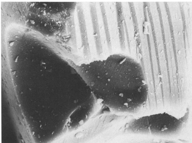
Fig. 2. Topography of carbon-silica adsorbent A 1 (SEM, \times 1000 ).
